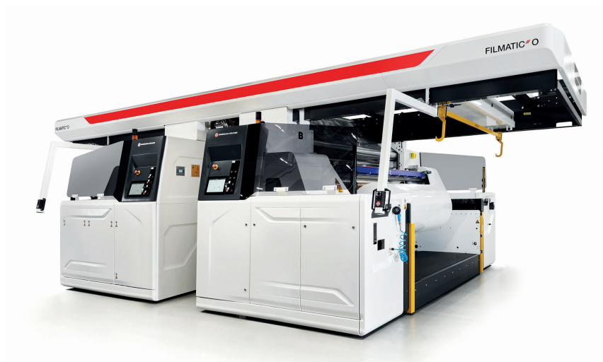
Fig. 3. The Filmatic II O contact winder in modular design was developed with a focus on optimal roll quality © W & H
